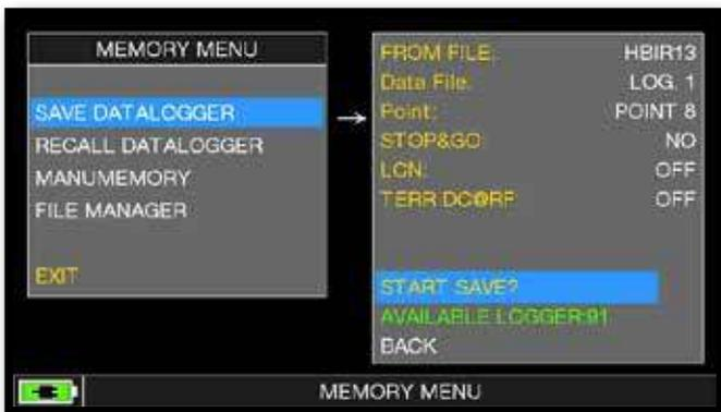
Set the parameters required. Touch "START SAVE" to create a new log file.
