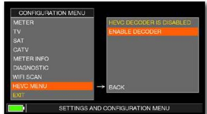
Touch "ENABLE DECODER" for enable the HEVC module.
