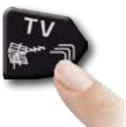
Press repeatedly to navigate into TV measures screens: Measures, Constellation, echoes and MER vs CARRIER.
