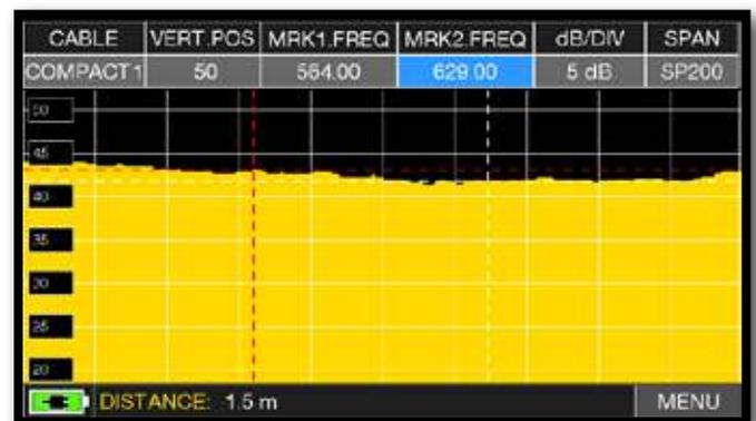
In the DISTANCE window, read the cable's mismatching value: example 1.5 m.
