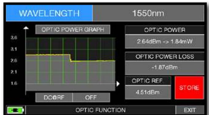
In the "OPTIC POWER LOSS" field, the optical attenuation value is displayed with respect to the stored value (Optic REF): for Example - 1.87 dBm.
